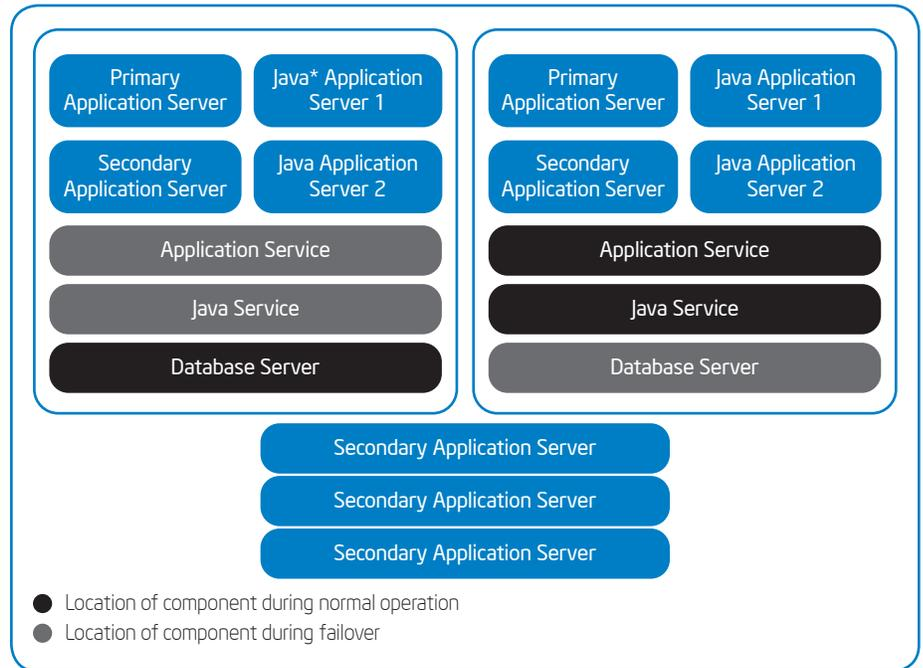
Figure 6. Two-socket servers running additional application server modules can be used to add incremental scale-out capacity to an existing large instance hosted on a clustered pair of four-socket servers.
