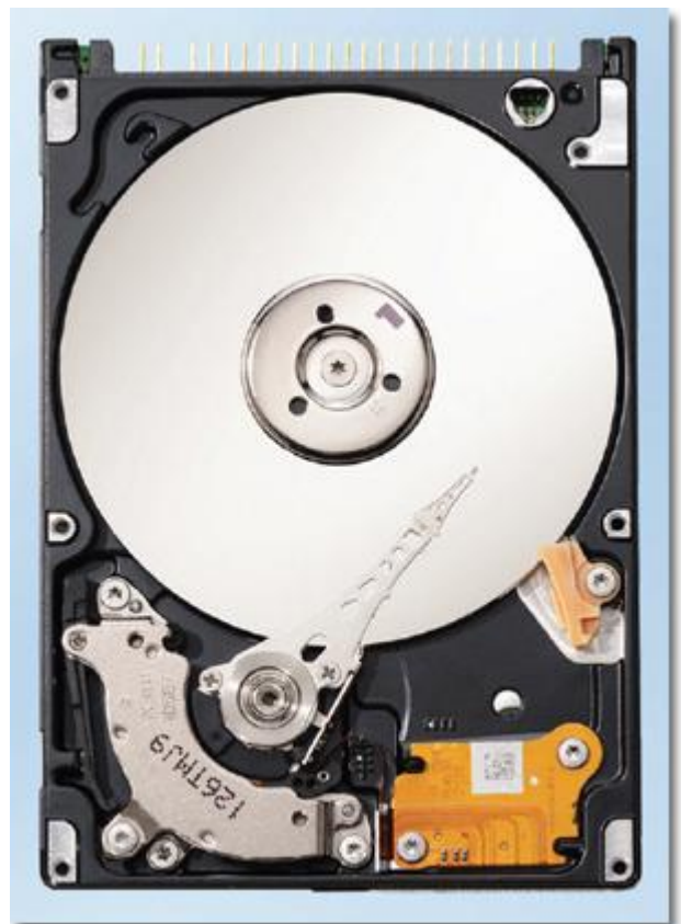
Figure 1: Data in a hard disk drive (HDD) is recorded on a rotating disk, which is vulnerable to sudden impact or temperature changes.
